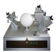
The circumference is determined by the CSM\* (Circumference and Sphericity Measuring System) ball test machine in combination with an ordinary PC and the related CSM- software package. The implemented "FIFA mode" runs an optimised test procedure and delivers the final results for the FIFA QUALITY PRO and FIFA QUALITY and FIFA BASIC categories. The CSM manual shows in detail the handling, calibration and measurements of the whole test system.
