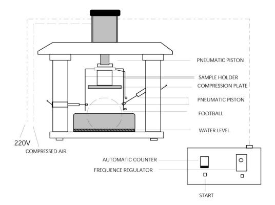
The machine must be capable of achieving a compression of 25% of any tested football's diameter. The piston shall be capable of a frequency of at least 40 compressions per minute. The receptacle shall be round and with a diameter of 30 cm  $\pm 2$ . It shall be filled with 2cm  $\pm 0.2$  of water. If a pressure plate is used for achieving compression, the diameter shall be 16cm  $\pm 1$ .
