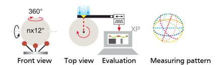
The radius is measured by the CSM machine in FIFA Mode. The circumference is calculated automatically as an average of 3 radii (calculated of 15 cycles each is used) x 2 x  $\pi$ , according to the FIFA definition avg. of 3 radii (45 cycles, split 3x15).
