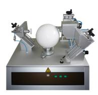
The circumference is determined by the CSM\* ball test machine in combination with an ordinary PC and the related CSM- software package. The implemented "FIFA mode" runs an optimised test procedure and delivers the final results for the FIFA QUALITY PRO and FIFA QUALITY and FIFA BASIC categories. The CSM manual shows in detail the handling, calibration and measurements of the whole test system.
